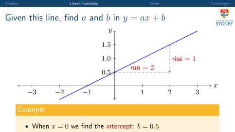
• The slope is  $a = \frac{\text{rise}}{\text{run}} = \frac{1}{2}$
